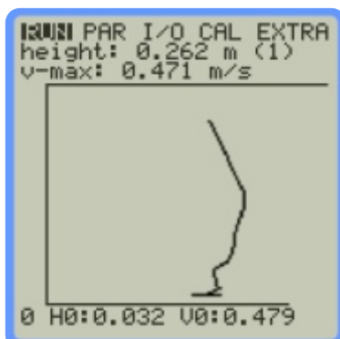
Flow profile indication on the display.
