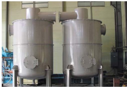
1st Mist & Dust Collector
