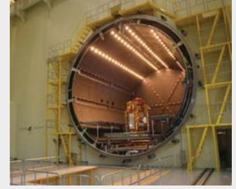
Cryogenic Vacuum Chamber Cryogenic temperature control unit for Vacuum chamber
