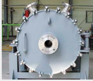
Waste Water Cooler
